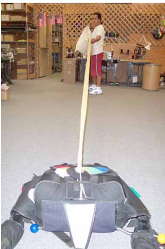
Notice that the Kevlar bridle on the left side of the container is scrunched up after you cock your drogue.
