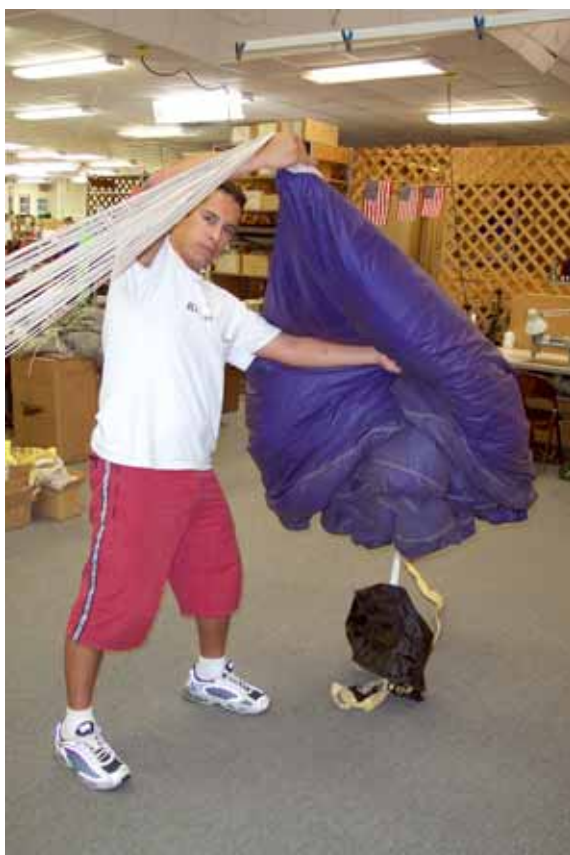
Neatly set canopy on floor. Carefull not to drop canopy on floor.
