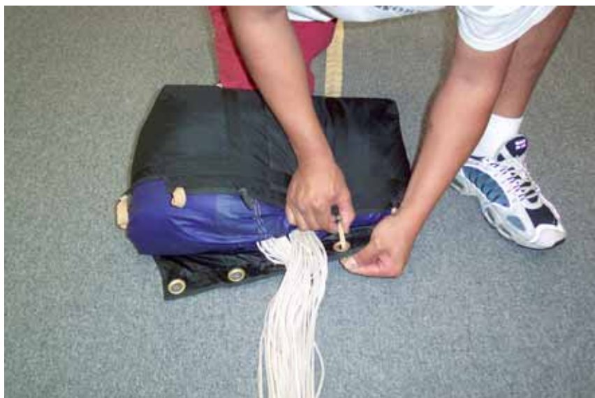
Secure D-bag with first 2 stows. Use tandem Tude stows here to reduce the chance of line dump.
